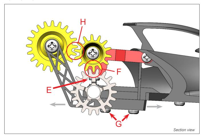
Adjusting the 2 screws (E) in the chassis (step 13) will change the center distance (F) of the idler gears and the rear wheels.
