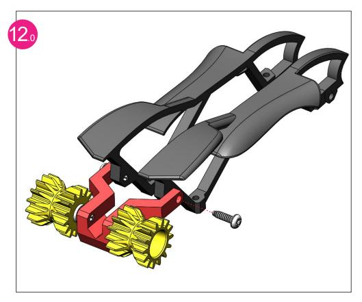
Install 2 screw ('A') into the chassis as shown. These will be used to adjust the center distance of the gears. More on that later.
