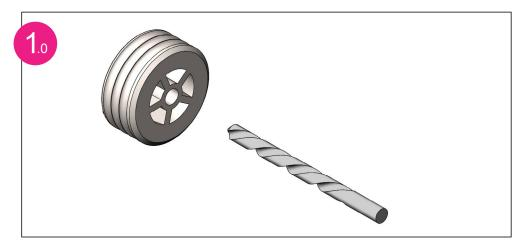
Ream the bore of the rear wheel with the drillbit. Ream both rear wheels.
