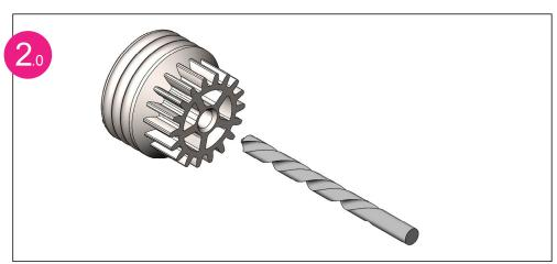
Ream the bore of the idler gear with the drillbit. **Ream both idler gears.**
