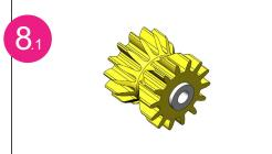
Insert two nylon bearings into the gear spool, one on each side.
