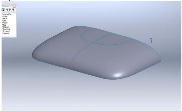
**Step 4** - The corner of the phone was completed by creating the surface that would wrap from the Boundary surface edge up to the top of the phone. I found the Loft tool gave me the surface I wanted. This was mirrored and then the entire end of the phone is mirrored about the Front Plane. This would give both ends of the phone.
