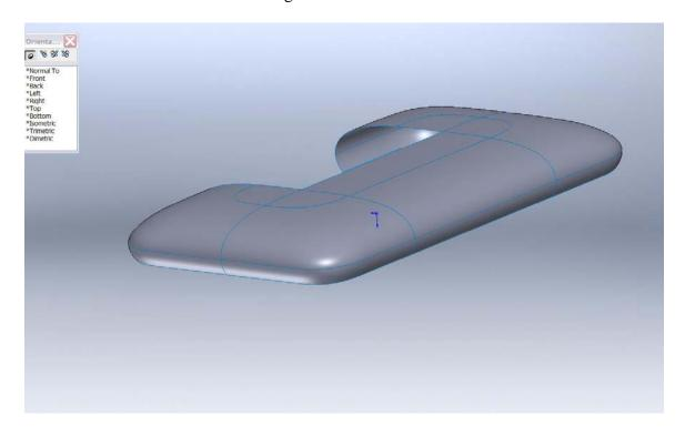
$\textbf{Step 6} \textbf{-} \textbf{To finish the body of the phone, I then selected the edges and used Fill Surface for the final planar surface. This was knitted to create a solid.$
