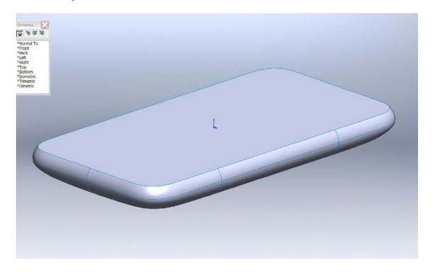
**Step 7** - From this point forward, I used the Apple 2D drawing to locate a surface to split the phone body to separate the upper chrome area and plastic lower body. All the details of the top lens areas and buttons were all done using the drawing as reference.
