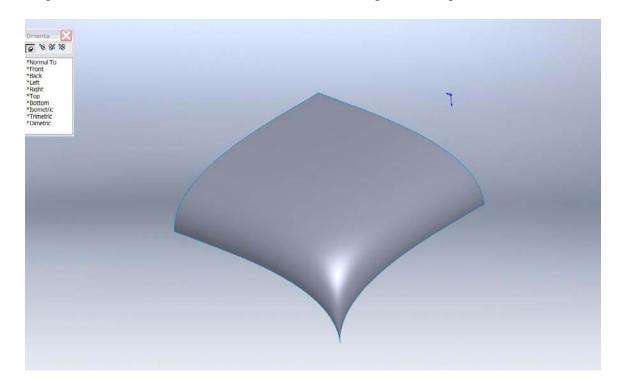
**Step 2** - The next step was to use the Boundary Surface tool and create the corner of the phone. The surface meets the newly trimmed Sweep and at the phone's widest point, which is also at the quadrant of the side and end view curve and allows the curve to end normal to the top plane. The Boundary Surface Direction one and two curves were all set to be normal to the curve and tangent to surface as appropriate. Pretty cool tool!
