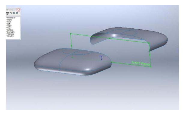
**Step 5** - I used the three edges of the 3 surfaces to extrude surfaces to fill in between the ends of the phone. These are then mirrored about the Right Plane to complete the bottom. These surfaces where then knitted together.
